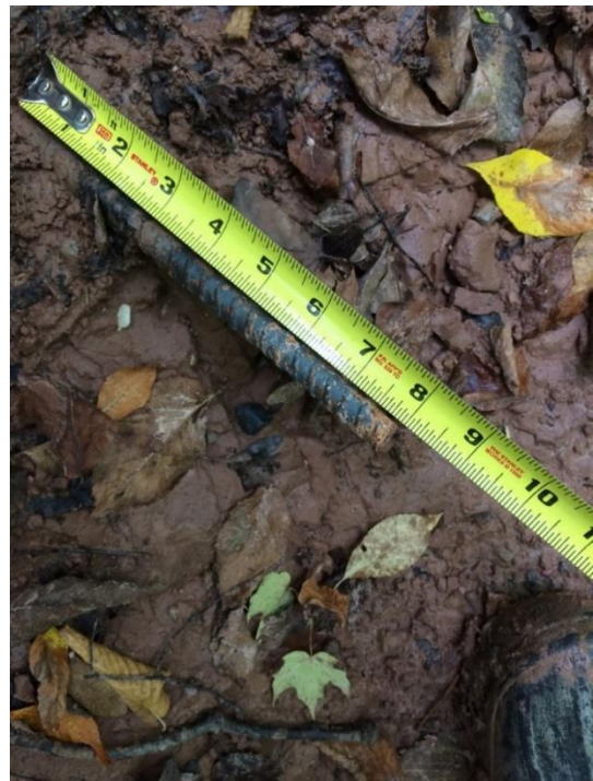
Figure 60. Erosion pin inserted into a streambank showing 8" of soil eroded after inspection in Kankapot Creek, Calumet County, Wisconsin.
