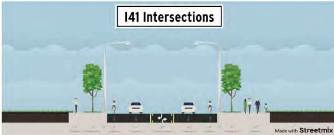
Figure B-2 Conceptual bicycle and pedestrian accommodations for I-41 crossings in the County Comprehensive Plan 2040
